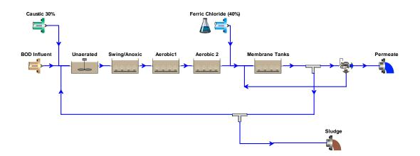
The swing/anoxic zone can be operated without aeration serving as an anoxic basin or aerated serving as an aerobic basin. This design approach maximizes operational flexibility.
